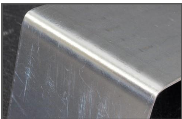
0.50 mm SIGMACLAD®60 annealed, bent 90° parallel to rolling direction (no cracking detected).
