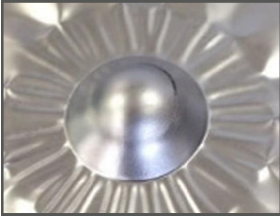
SIGMACLAD® Erichsen Cup height Test Sample
