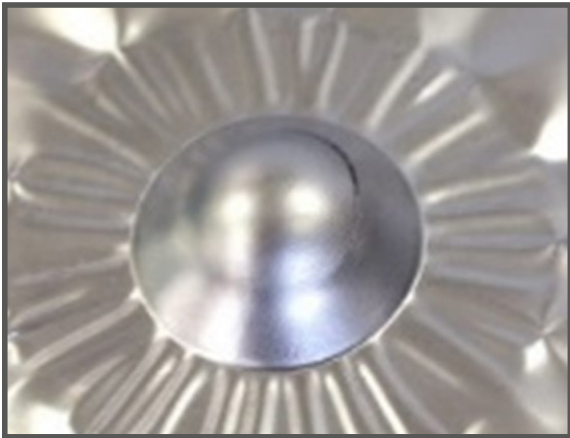
SIGMACLAD® Erichsen Cup height Test Sample
