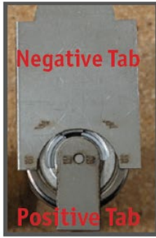
21700 Cell Laser Welded
