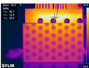
Thermal Image after 5 minutes discharge with 0.250 mm Nickel/0.250 mm Copper welded assembly endplate. Point temperature 54.5 °C
