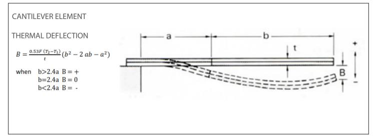
A reverse welded cantilever element of B1 thermostatic bimetal is available with section a = 1" and section b = 2". Find the thickness required to give a deflection of -0.026" from 50°F to 150°F.
