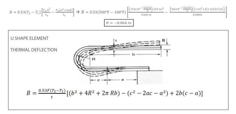
A strip of reversed welded P675R thermostatic bimetal is formed into a U-shape with the following dimensions: c = 0.5", b = 2", a = 1", R = 0.25". Find the thickness of material required to give a deflection of 0.15" from 50°F to 150°F.
