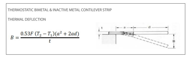
A strip composed of 1" of B1 thermostatic bimetal butt welded to 1-1/2" of a thermally inactive material is to be used as a cantilever. Using 0.030" thick material, find the deflection produced by changing the temperature from 50°F to 200°F. The flexivity of B1 between 50°F to 200°F range is 150 x 107(in/in)/°F.
