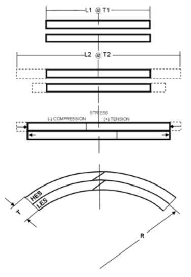
1. Two metal strips of identical length (at a given temperature) having high and low coefficients of thermal expansion.
