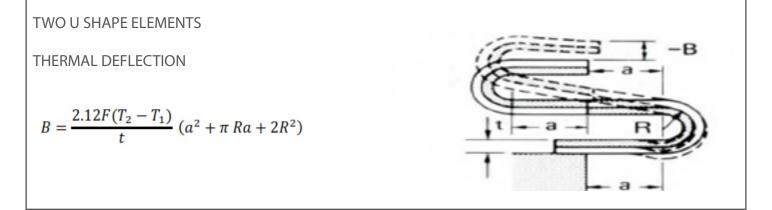
A reverse welded thermostatic bimetal U-shape is made of 0.20" thick B1 with 0.5" radii and section a = 1". Find the deflection from 50°F to 200°F. The flexivity of B1 is 150 x 10<sup>-7</sup>(in/in)/°F.
