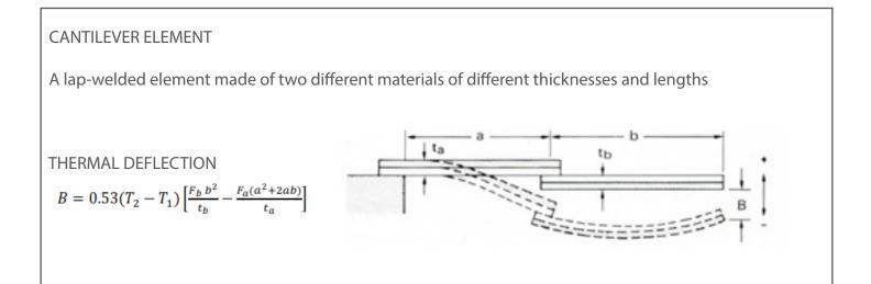
A reverse lap-welded element is made of E4 and B2. The E4 is  $0.040'' \times 1''$  (section a); the B2 is  $0.020'' \times 0.5''$  (section b). Find the deflection through a temperature change from  $100^{\circ}$ F to  $500^{\circ}$ F
